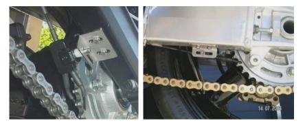
The PRO-OILER's nozzle system is critical for efficient and accurate delivery of oil to the chain.
